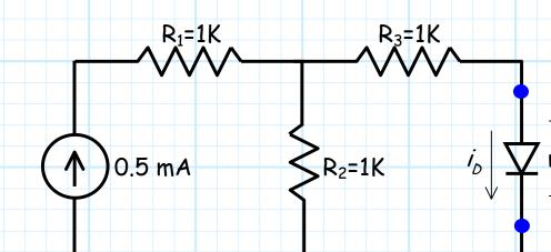
Using the CVD model, let's estimate the voltage across, and current through, the junction diode.
